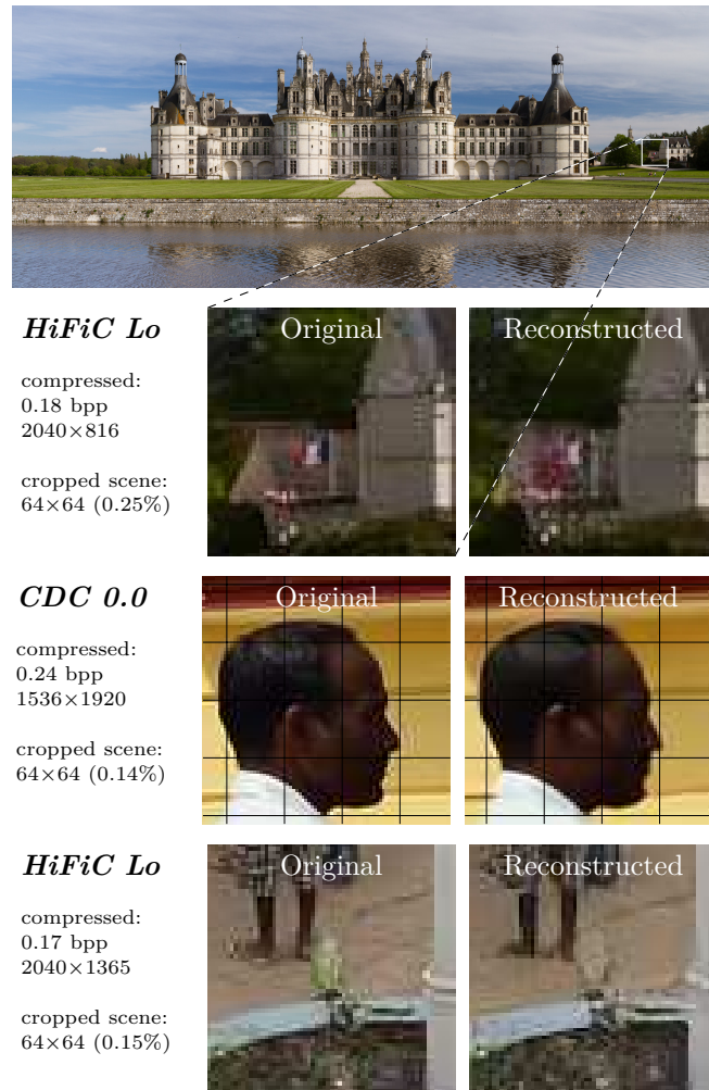
Figure A.4: Category GEOMETRY: Reconstructions contain geometric transformations, such as translation, rotation, scaling, and shearing, including shifted shapes and dissolved contours. (The top image illustrates the level of detail at which miscompressions occur. A grid was added to the middle crop.)
