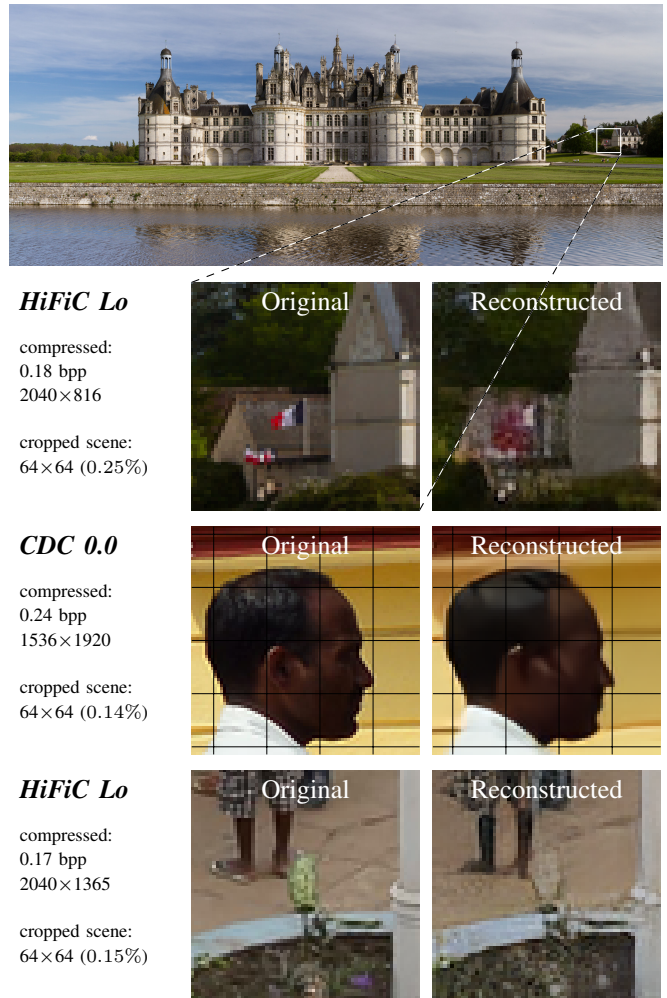
Fig. 4. Category GEOMETRY : Reconstructions contain geometric transformations, such as translation, rotation, scaling, and shearing, including shifted shapes and dissolved contours. (The top image illustrates the level of detail at which miscompressions occur. A grid was added to the middle crop.)
